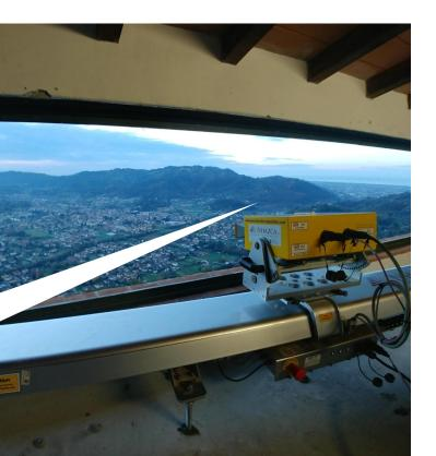
Synthetic Aperture Radar Interferometry (InSAR) is a valuable technique for estimating surface deformation processes using sensors installed on satellite (A-DInSAR) and ground (TInSAR) platforms.
